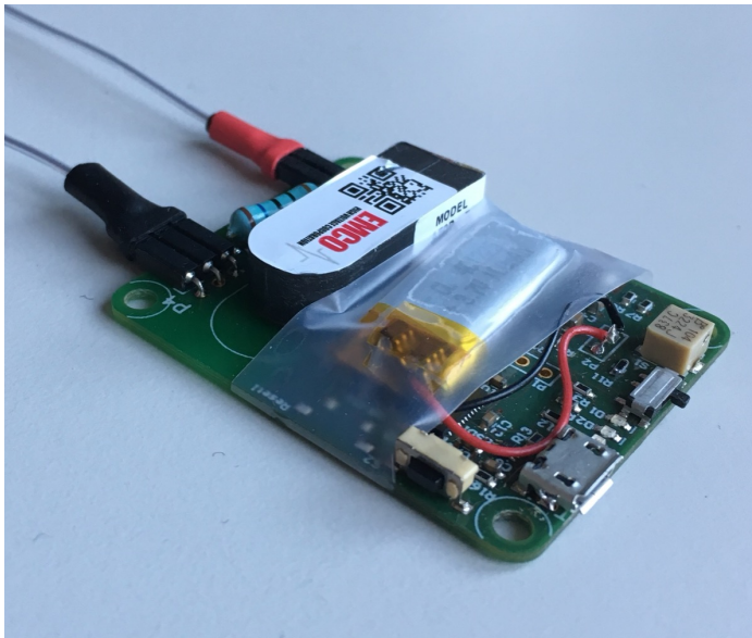
Miniature 1 channel 5 kV 1 Hz power supply: 16.0 g
